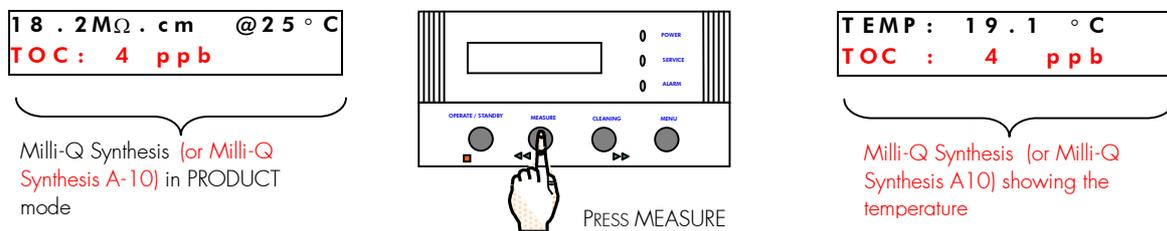
The temperature will be displayed for about 10 seconds. The LCD will return to the resistivity display.
